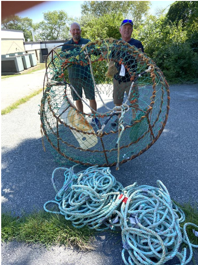
The snow crab pot and rope removed from Ruffian, #3530, off northeast Florida on 6 January 2017. The gear was dragged down from Canada, some 1,200 miles. The pot is of heavy construction and weighs about 120 lbs.
